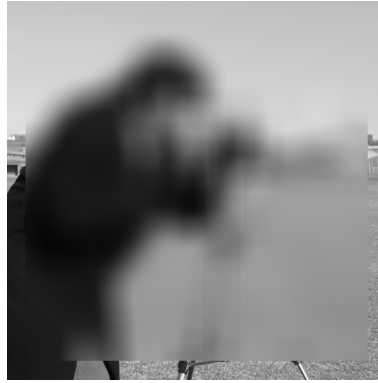
Figure 1.11: Illustration of a simple convolution filter, a mean filter of size 25 \times 25 . One can see the sides of the image have not been filtered.
